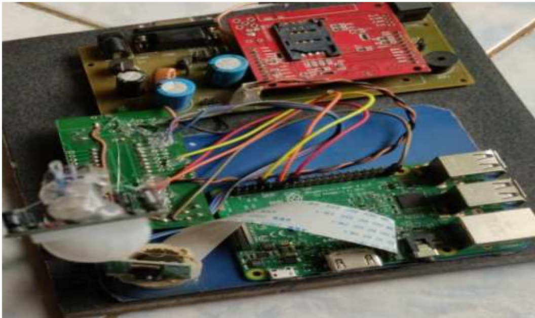
Fig. 8 Home Security System Using Raspberry Pi
